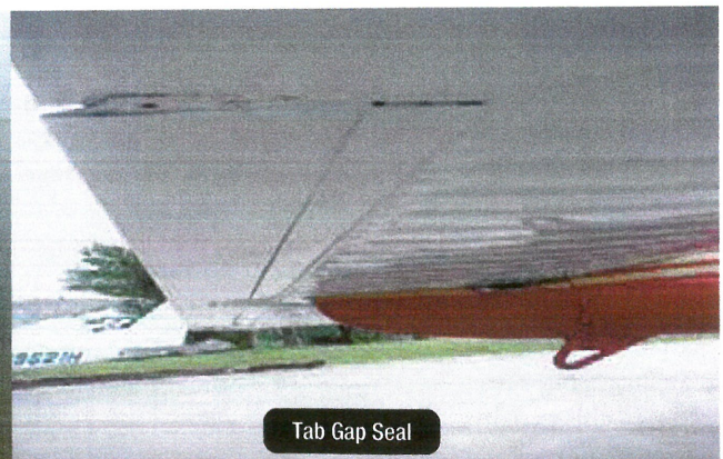
Figure 3-15. Gap seals promote the smooth flow of air over gaps between fixed and movable surfaces.
