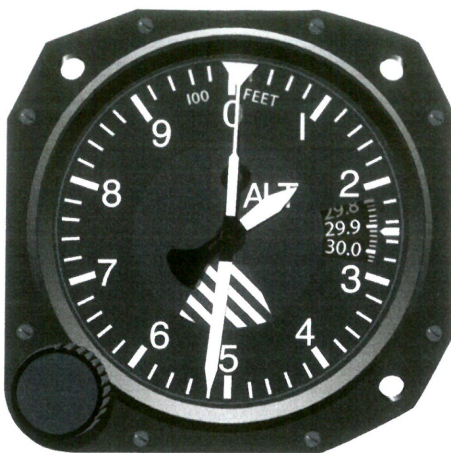
Figure 1-3. An airplane's altimeter is an aneroid barometer.
