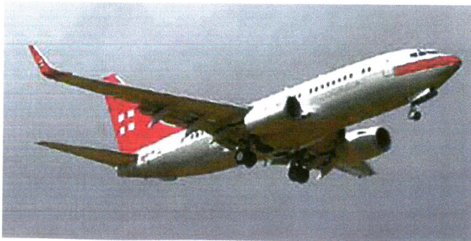
Figure 3-12. A winglet reduces induced drag caused by air spilling off of the wingtip.
