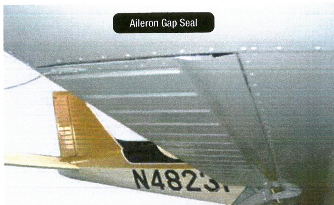
Figure 3-15. Gap seals promote the smooth flow of air over gaps between fixed and movable surfaces.
